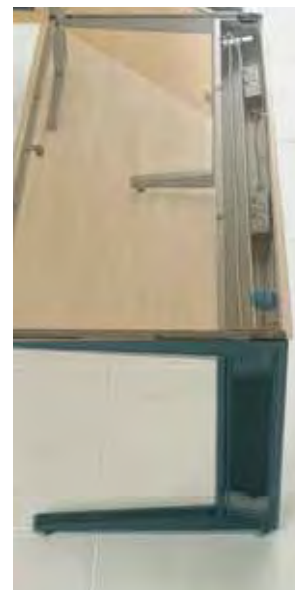
Fig 2: Power unit & cables in Directiv cable management system. Showing sliding desktop closed.
